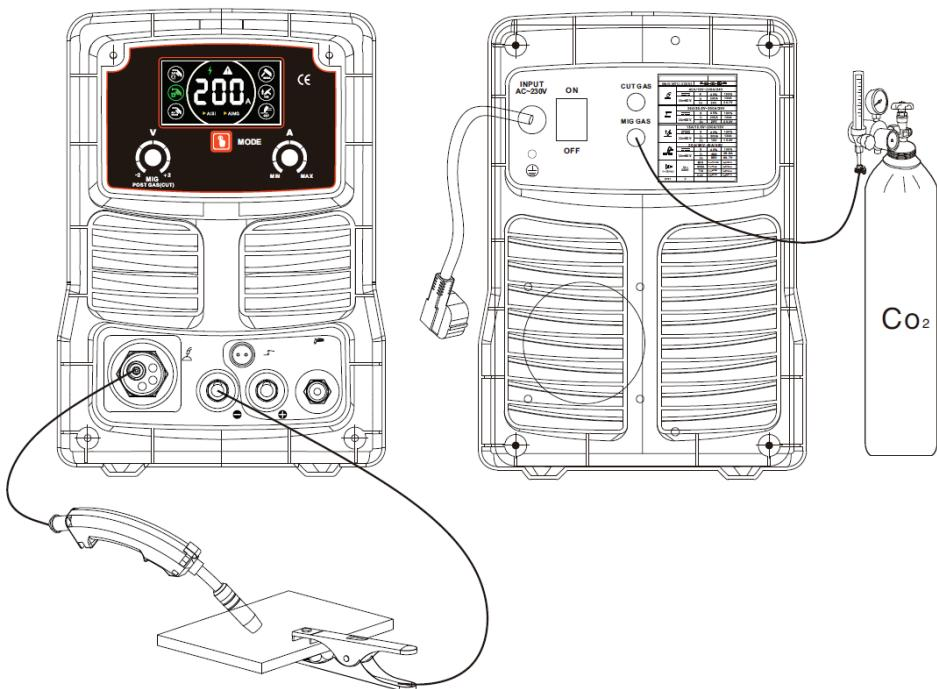
When you open the door to put MIG solid wire (GAS: CO<sub>2</sub>), please see the following connection, it should be connect with positive pole “+”
