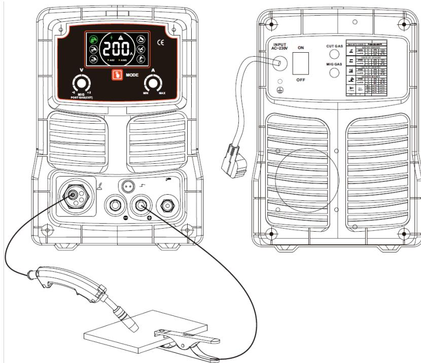
When you open the door to put MIG flux-cored wire (NO GAS) , please see the following connection, it should be connect with negative pole “—”
