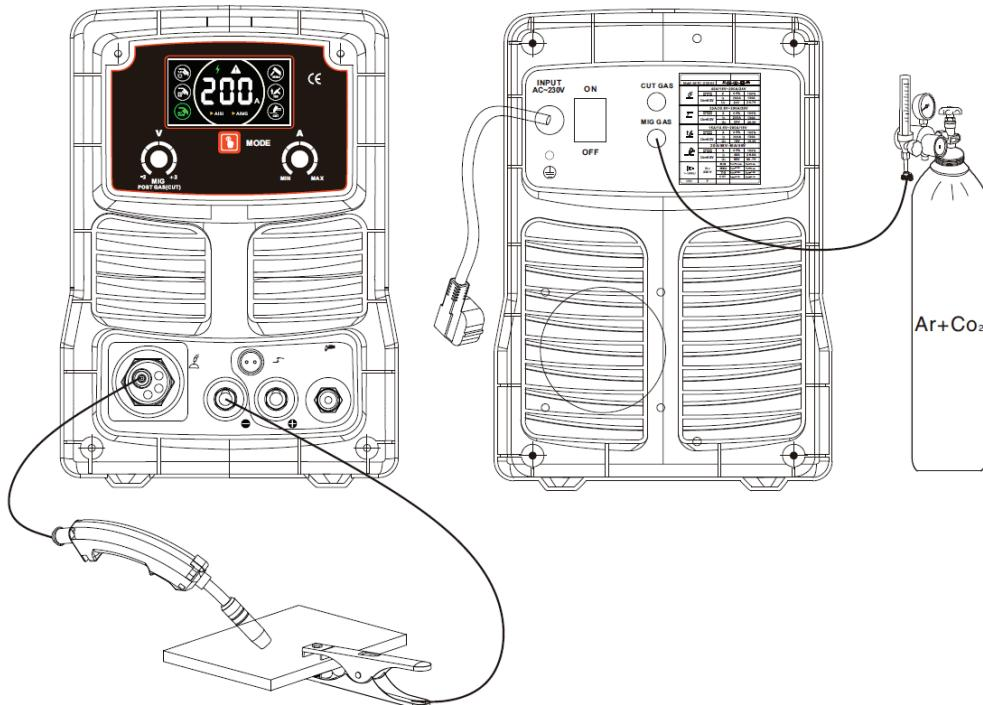
When you open the door to put MIG solid wire (GAS:Ar+ CO<sub>2</sub>), please see the following connection, it should be connect with positive pole“+”
