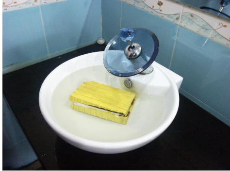
Put the uncovered cell into water
