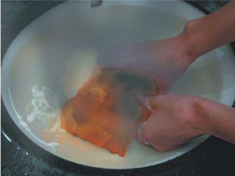
Put the burning battery into water
