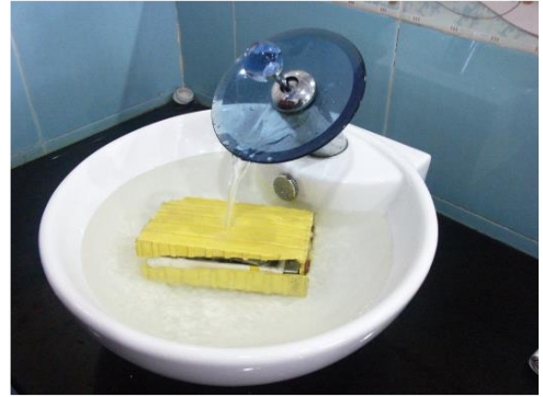
Uncovered cell gets fully soaked by water
