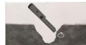
If you do not receive a response from inside the hole or the soil/plug that was removed, the object is likely deeper in the Ground or deep inside the plug-beyond pinpointing range. Sweep with your ground search detector again to confirm where the object is.
