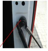
Secure circlips to stud in order to hold EZDown in place at the upper and lower stud
