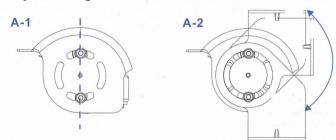
A-1. Recommended guide line for assembling sunvisor. A-2. User can adjust the installation angle.
