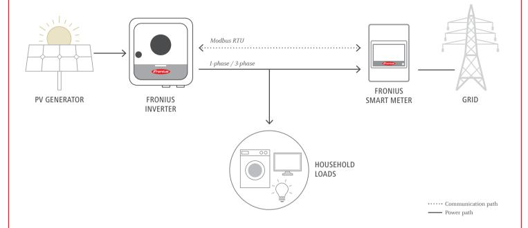
The Fronius Smart Meter is compatible with all inverters with an RS485 interface (Modbus RTU). The Fronius Smart Meter can be retrofitted at any time together with the Fronius Datamanager 2.0 in inverters that have already been installed.
