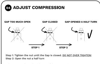
! The top nut adjusts the tightness of the compression system.
