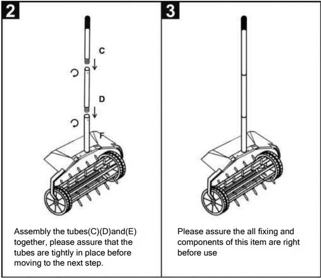
Assembly the tubes(C)(D)and(E) together, please assure that the tubes are tightly in place before moving to the next step.
