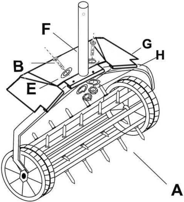
1.Using(B) part screw fittings screw the head(A) to the tube(F).Please make sure all fittings are security
