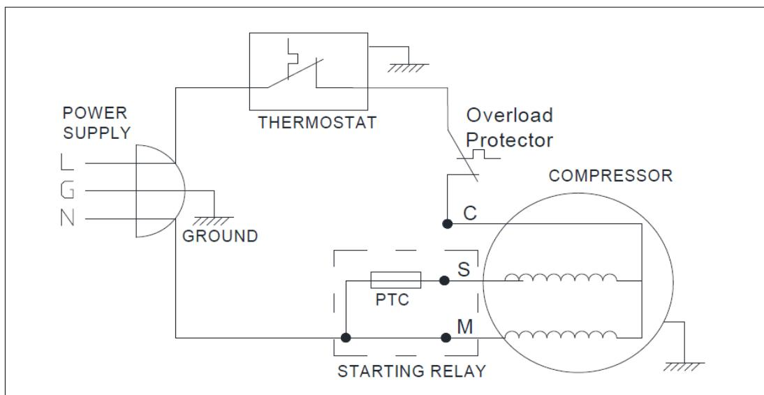
*Note: The compressor may not be equipped with the running capacitor according to actual compressor model using.*
