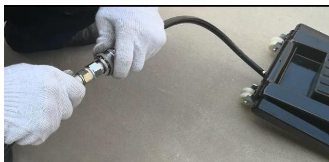
Turn the lift upside down, Turn on the power unit, Insert the plug into 220V/50Hz socket, press the "Up" button of remote control to rise to the top, press the "Down" button to fall to the ground, repeat 2 or 3 times, discharge the gas in the pipeline and its cylinder (no crawling state when the cylinder rises or falls), and then turn over the lift.
