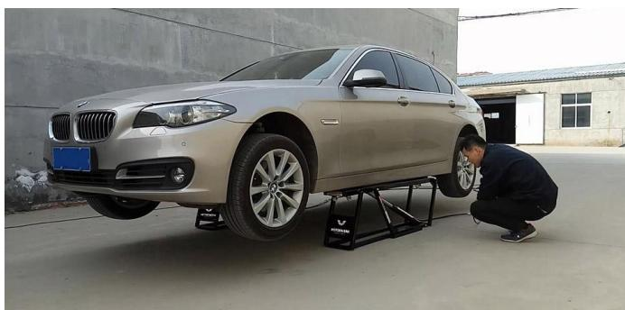
Press the "Down" button to fully lock the mechanical lock and start maintenance work
