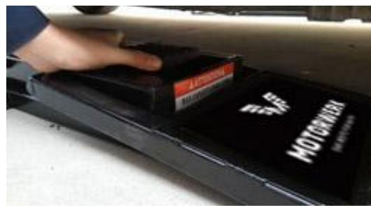
The bottom of the lifting frame is equipped with universal wheels, which can be pushed to the bottom of the vehicle from front to back, from left to right.
