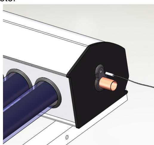
When install, please put the temperature sensor through into the small hole that is "O" appearance, "8" type circle.
