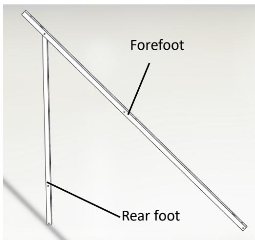
2. mounting the bracing, connect the bracing to the fore foot and the rear foot with bolt M8\*25 to fixed.
