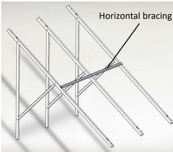
5. Aligned The two holes of the cross brace and connect with bolt M8 \* 25.
