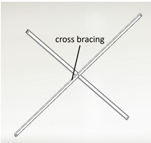
6. Mounting the cross brace, fix the two pairs of the cross brace on the rear foot with bolt M8\*25.
