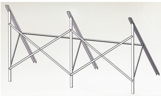
7. Mounting tail bracket, connect the tube row to the fore foot with bolt M8\*25 to fixed.
