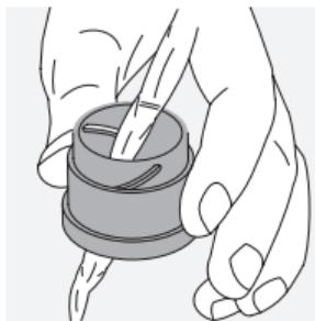
The housing is best cleaned with a soft, moist cloth (please do not use the lens-cleaning cloth for this). If it is very dirty (e.g. with sand), the twist-in eyecup can be completely unscrewed for very easy cleaning.
