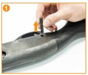
With the pump arm fully forward and the safety on, remove the larger diameter OEM receiver pin (the pin closest to the stock) by lightly tapping the pin out with a proper hammer and punch.
