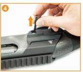
Remove the remaining OEM receiver pin by lightly tapping the pin out with a proper hammer and punch.
