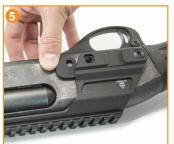
Insert our two included shims into the space between the optic mount and receiver on both sides. Make sure the shims are orientated so that it follows the optic mount's contour. From the left side of the optic mount, install our smaller diameter Torx receiver pin. Lightly tapping the pin through may be required.
