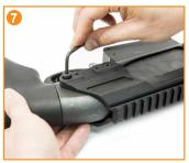
Install and hand tighten the Torx receiver pin with the included tool until the Torx head is flush with the optic mount. Apply 20 In-lbs of torque to both Torx receiver pins.
