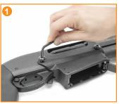
With the pump arm fully forward and the safety on, remove the threaded Hex receiver nut and pin holding the magazine well's rear tang in place using a 5/32 Hex key. Lightly tap the pin out with a proper hammer and punch.
