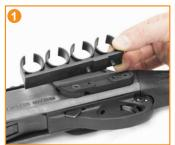
Place and hold the shot shell carrier on the left side of the mount aligning the mount's screw holes with that of the carrier's. The carrier should be orientated so that it overlaps the receiver only and not where the stock meets the receiver.
