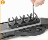
Insert the included Hex screws and tighten using the included tool. Recommended torque value is 15 In-lbs.
